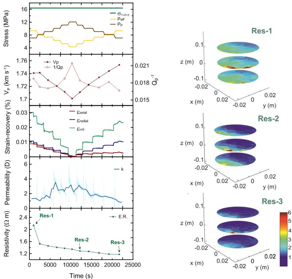
Figure 2. Left, geophysical monitoring and hydro-mechanical evolution of Utisira sand during the brine flooding test. Right, 3D-ERT of the sample in three test steps (Res-1, Res-2 and Res-3).
